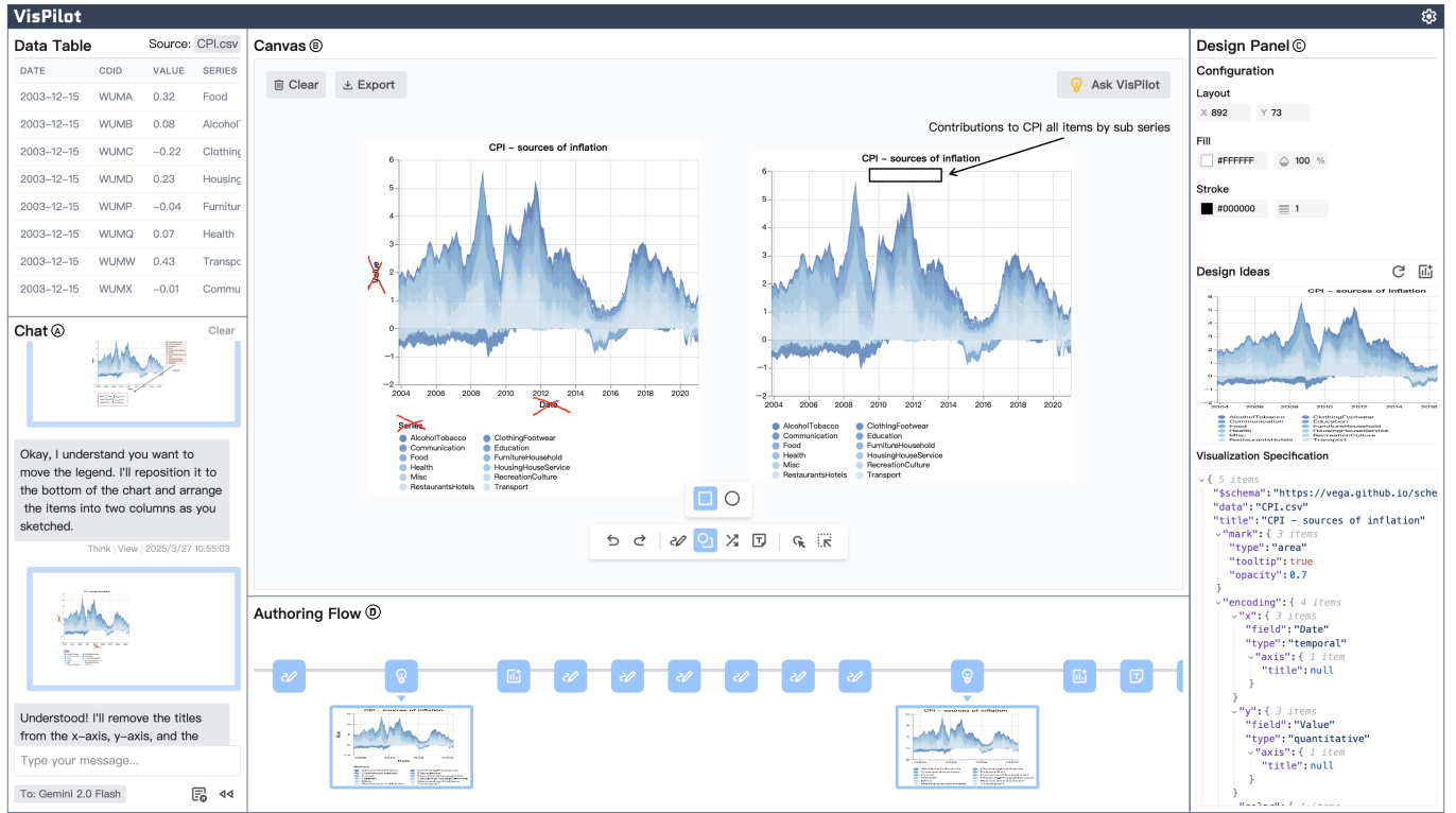
Fig. 5: The interface of VisPilot includes four components: (A) Chat Interface, (B) Free-drawing Canvas, (C) Design Panel, and (D) Authoring Flow.
